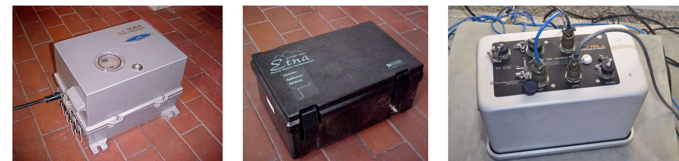
Fig. 1 (Left) SM-10B RION, (center) ETNA Kinemetrics, (right) 130-SMA RefTek accelerographs implemented in REDACIS
